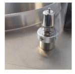
Indirect heating with low-pressure steam generated by the water in the jacket: safe and easy operation thanks to pressure gauge, safety valve and compensating valve.
