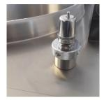
Indirect heating with low-pressure steam generated by the water in the jacket: safe and easy operation thanks to pressure gauge, safety valve and compensating valve.
